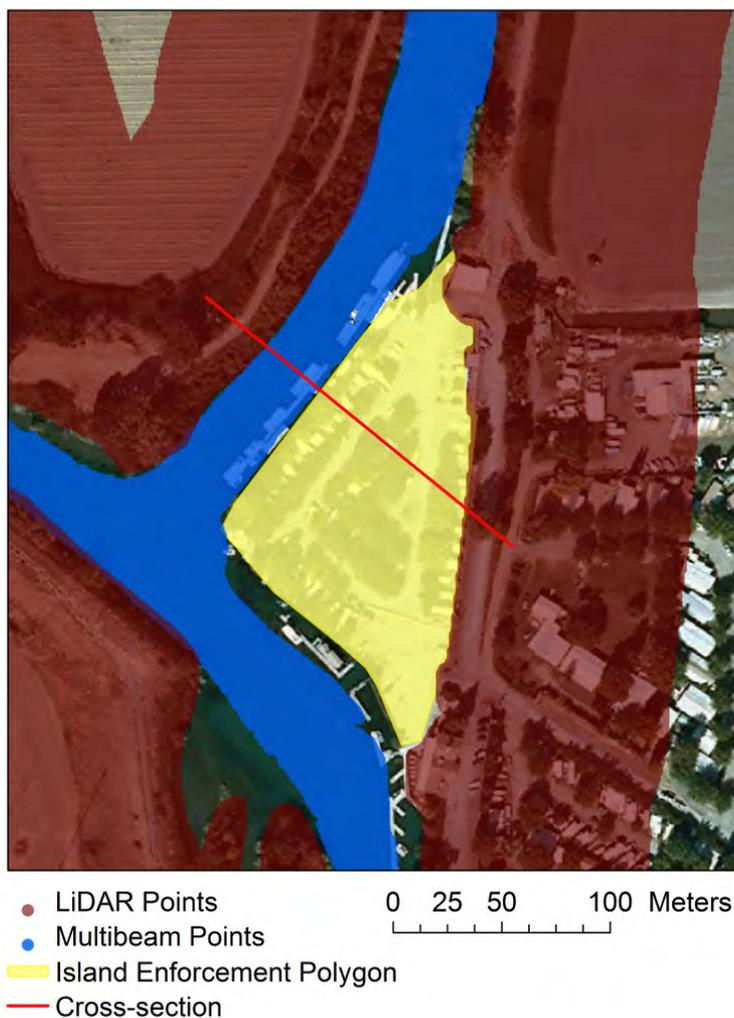
**Figure 6-8 Delineation of an Inhabited Island Using Bounds of a Polygon as a Hard Constraint**
