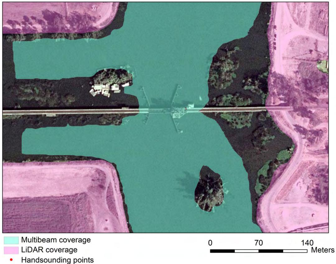
Figure note: The gap in the west side of the figure is due to an island with no LiDAR returns. The gap in the east is more complex, involving shallows, small islands, and structures. In this case, there were few recent hand soundings to support interpolation near the islands.
