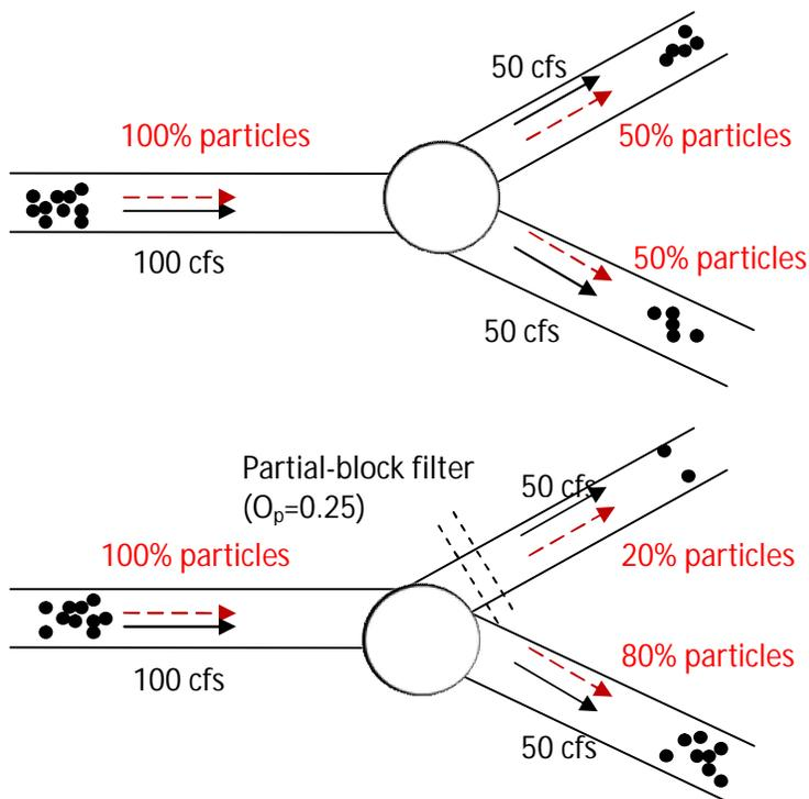
**Figure 5-1** Flow and particle fluxes at two equal-branch junctions, with a partially-block filter set on one branch (Solid arrows depict flow; dashed arrows depict particle fluxes). The particle amount in the plot is for illustration only, and is not the actual amount.
