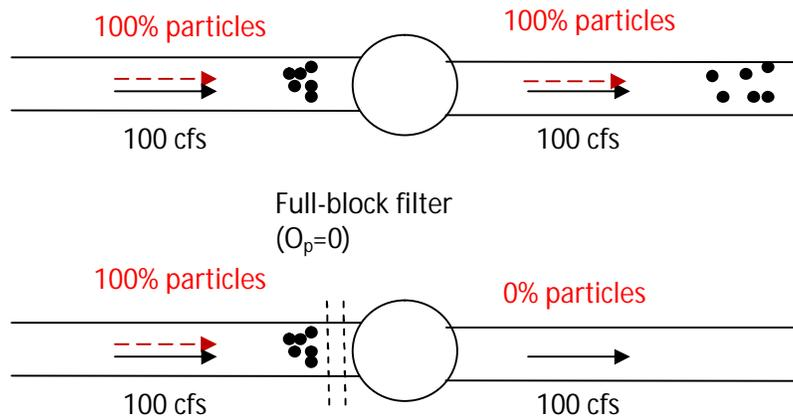
**Figure 5-4 Flow and particle fluxes w/o and with a full-block filter set before the particle-entering node (Solid arrows depict flow; dashed arrows depict particle fluxes).**
