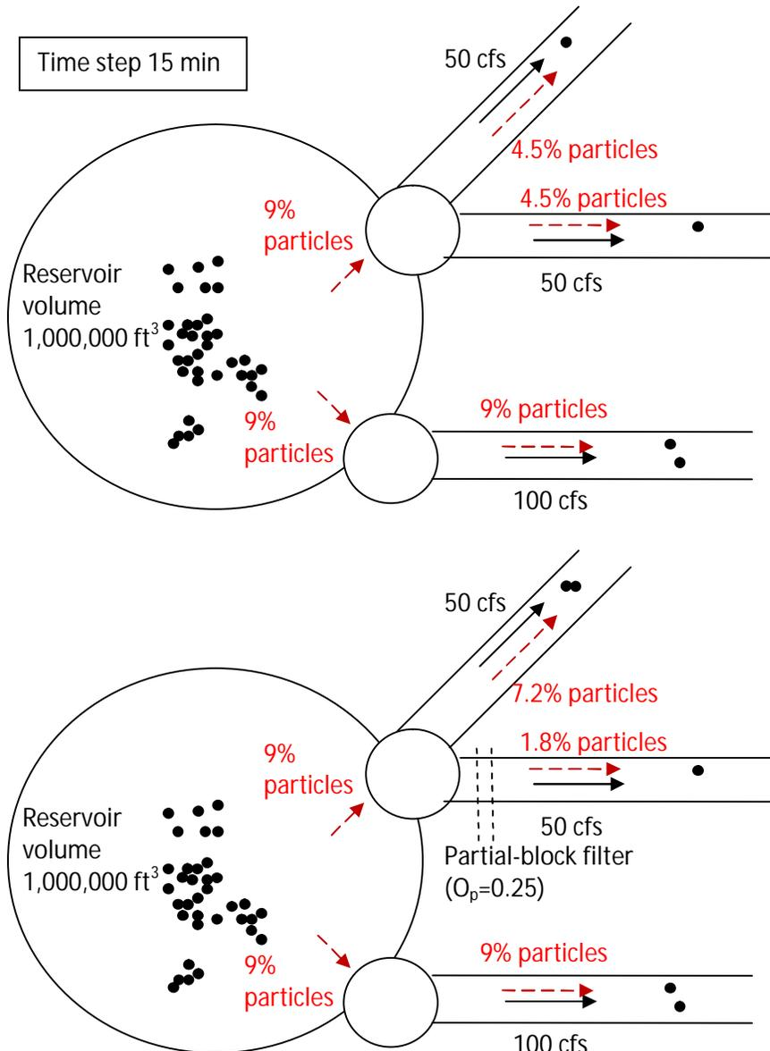
Figure 5-3 Flow and particle fluxes w/o and with a partial-block filter set after the particle-entering node in grid with reservoir (Solid arrows depict flow; dashed arrows depict particle fluxes).
