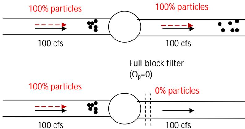
**Figure 5-2** Flow and particle fluxes without and with a full-block filter set after the particle-entering node (Solid arrows depict flow; dashed arrows depict particle fluxes).
