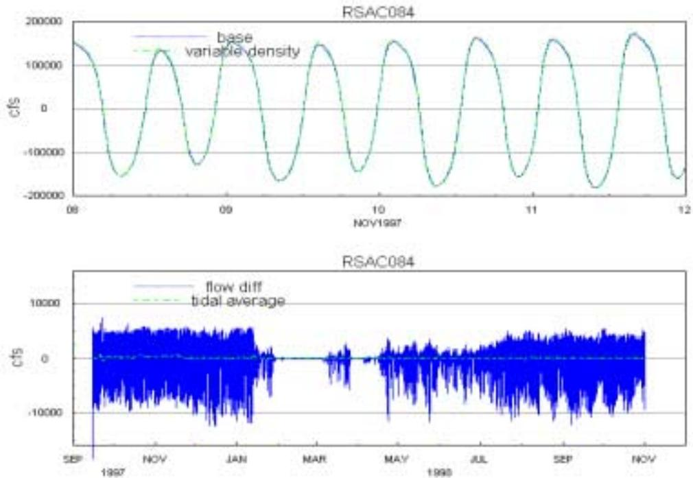
Figure 6-3: (Top) Flow near Sherman Lake. (Bottom) Difference between cases (variable density minus base) and its tidal average.
