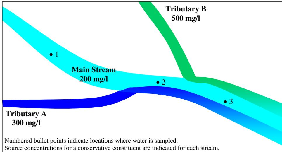
**Figure 14.1: Conceptualization of a Stream with Two Tributaries.**
