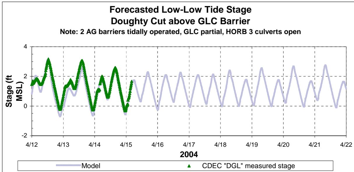
**Figure 8.3: Example of Forecasted Water Levels Using DSM2.**
