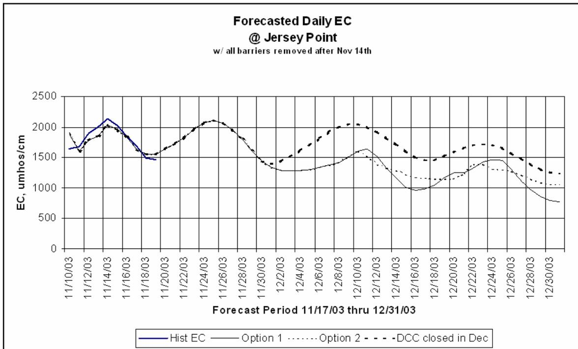
**Figure 8.2: Example of Forecasted Water Quality Using DSM2.**
