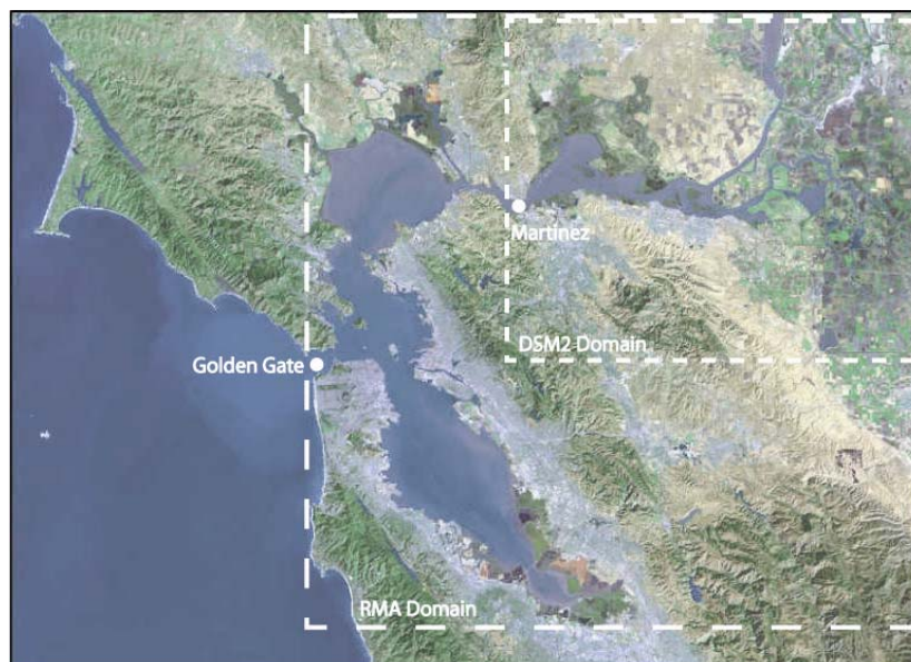
Figure 5.2: Map of San Francisco Bay and the Delta with RMA and DSM2 Model Boundaries. (Satellite image from US Geological Survey).
